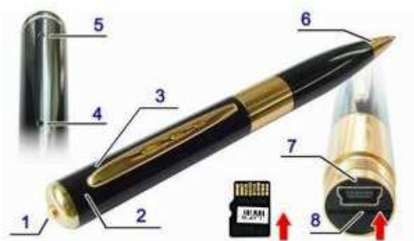
1: operation button 2: camera 3: MIC 4: reset button 5: status indicator 6: ball-point pen 7: USB 8: TF card Socket
